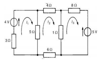
The mesh currents I1, I2 and I3 are shown in Figure Using Kirchhoff's voltage law: For loop 1, (3 + 5) I1 -I2 = 4 ....(1) For loop 2, (4 + 1 + 6 + 5) I2 -(5) I1 -(1) I3 = 0....(2) For loop 3, (1 + 8) I3 -(1) I2 = 5- ....(3) Thus
