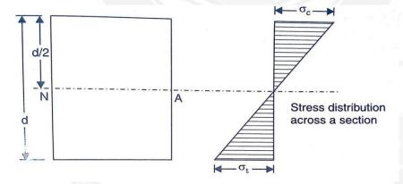
**Problem 2.13.** A steel plate of width 120mm and of thickness 20mm is bent into a circular arc of radius 10m. Determine the maximum stress induced and the bending moment which will provide the maximum stress. Take  $E = 2 \times 10^5 N/mm^2$ .
