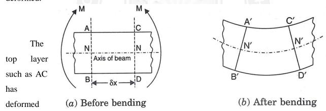
to the shape A'C'. This layer has been elongated. It is clear that some of the layers have been shortened while some of them are elongated. At a level between the top and bottom of the beam there will be a layer which is neither shortened nor elongated. This layer is known as neutral layer or neutral surface.
