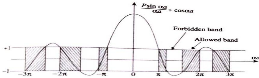
Fig. 5. 13 A plot of  $\alpha a$  versus  $\left(\frac{P \sin \alpha a}{\alpha a} + \cos \alpha a\right)$
