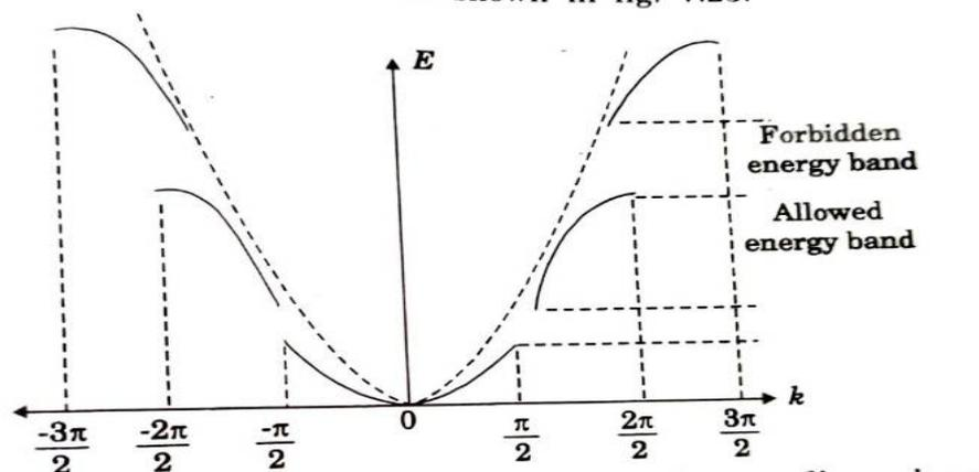
Fig5.14 Plot of energy Vs. wave vector in one dimensional lattice
