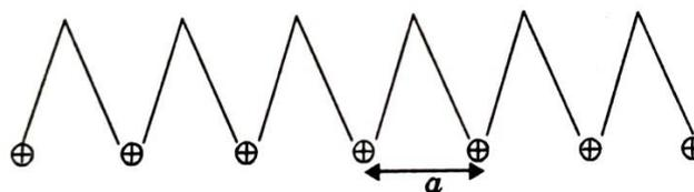
Fig. One-dimensional periodic potential distribution on electron in crystal lattice
