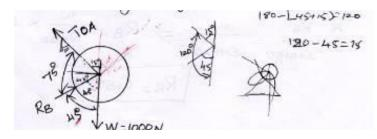
No of force is 3, so by using Lami's theorem
