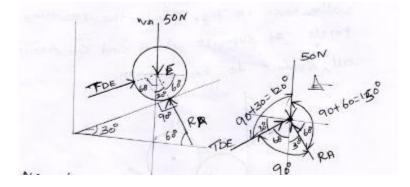
No of forces is three, apply Lami's Theorem
