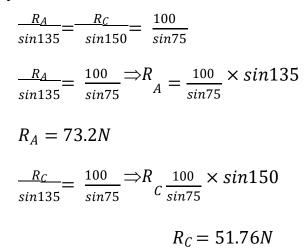
11.A Ball weighht120N in a right angle groove as shown in fig. The sides of the groove are inclined at an angle of 30°*and* 60°to the horizontal. If all the surface are smooth,then determine the reaction RA&RC at the point of contact
