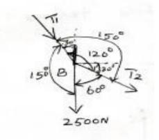
By Lami's Theorem  $\frac{TBA}{sin60} = \frac{TBC}{sin150} = \frac{Z500}{sin150}$   $\frac{TBA}{sin60} = \frac{2500}{sin150}$   $T_{BA} = \frac{2500}{sin150} \times sin60$  T1 = 4330.13 N  $\frac{T_{CB}}{sin150} = \frac{2500}{sin150}$
