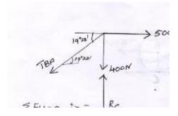
$\sum FH = 0 \quad \rightarrow + \quad - \leftarrow$   $\sum FH = -T_{BA}cos19^{\circ}28' + 500=0$   $-T_{BA} = cos19^{\circ}28' = -500$   $-T_{BA} = \frac{-500}{cos19^{\circ}28}$   $-T_{BA} = 530.31N$   $\sum FV = 0 \downarrow - \uparrow +$   $-400+R_c - T_{BA} \sin 19^{\circ}28' = 0$   $R_c = T_{BA}sin19^{\circ}28' + 400 = 530.31 \times sin19^{\circ}28' + 400$
