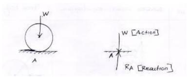
Consider a Ball placed on a horizontal surface shown in fig. The self weight of the ball (w) is acting vertically downwards through its centre of gravity. This force is called Action.
