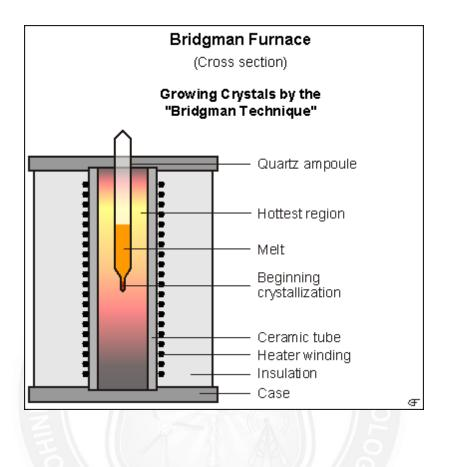
• It consists of a vertical cylindrical container made by platinum or quartz, tapered conically with a point bottom.
