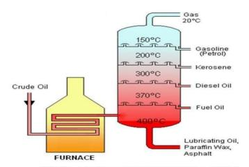
Purified crude oil is heated to 400°C in an iron retort. The oil gets vapourised. The hot vapours are passed up a 'fractionating column'. The fractionating column is a tall cylindrical tower containing a number ofhorizontal steel trays at short distances. As the vapours go up they become cooler and get condensed at different trays.
