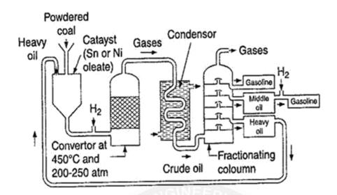
During this process, hydrogen combines with coal to form saturated higher hydrocarbons which further decomposes to yield low – boiling liquid hydrocarbons (crude oil) while passing through a condenser.
