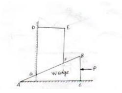
A wedge is a piece of wood or metal, usually of a triangular (or) trapezoidal shape in cross section used for Lifting Loads (or) for slight adjustment like tightening keys for shift
