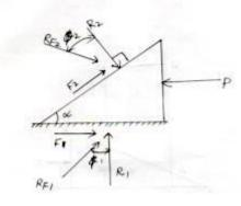
Normal force and Frictional force are combined to a single resultant force ' $R_F$ '  $R_{F1} \& R_{F2}$  are drawn on wedge
