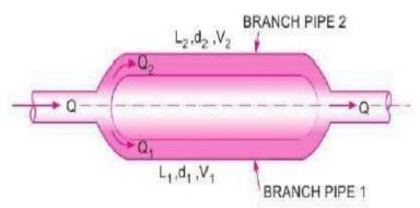
It is analogous to parallel electric current in which the drop in potential and flow of electric current can be compared to head loss and rate of discharge in a fluid flow respectively.
