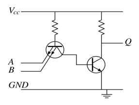
TTL inputs are the emitters of a multiple-emitter transistor. This IC structure is functionally equivalent to multiple transistors where the bases and collectors are tied together. The output is buffered by a common emitter amplifier.
