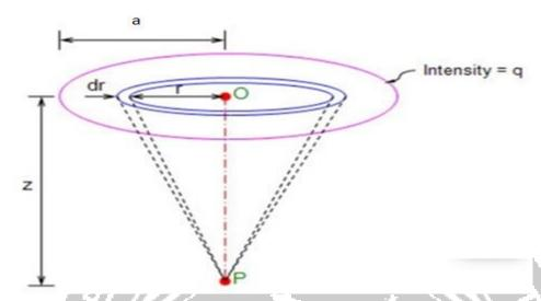
The Boussinesq equation for vertical stress due to a point load can be extended to find the vertical stress at any point beneath the centre of a uniformly loaded circular area.
