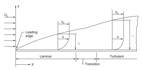
Figure 3.1.1 Boundary Layer Development (flat-plate)
