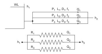
$\mathbf{Case}\ (i)$  The head drop between locations 1 and 2 are specified: The total flow can be determined using
