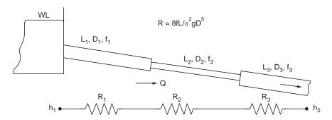
Figure 3.19.1 Equivalent circuit for series flow
