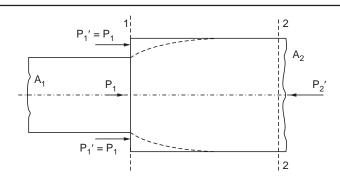
Applying conservation of momentum principle to the fluid between section 1 and 2, and denoting the actual pressure at section 2 as  $P_2$ ,
