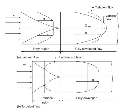
Figure 3.3.1 Boundary layer development (pipe flow)
