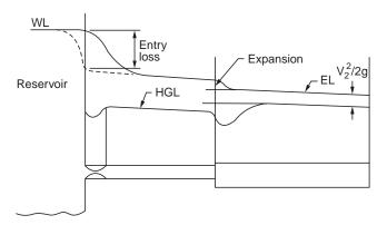
Figure 3.15.1 Energy and Hydraulic grade lines
