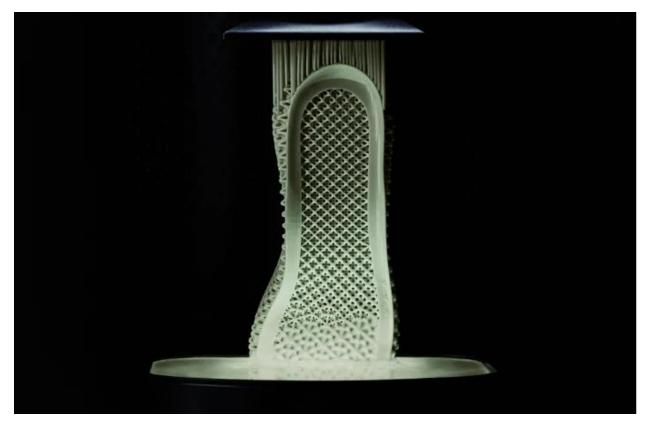
For the means of producing around 100.000 pairs, Adidas partnered with a company named Carbon. Carbon is a young company which invented 'Digital Light Synthesis,' a 3D printing technology similar to DLP, but improved. DLS is special for continuous printing thanks to the continuous motion of the build plate elevator. Standard DLP machines pause at a certain height until the layer is finished, but Carbon's 3D printers continuously raise the build plate.
