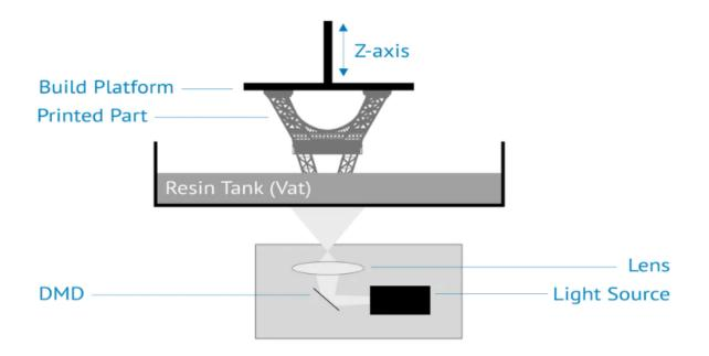
The digital light projector is the light source of a DLP 3D printer. The DMD (Digital Micro mirror Device) is a component which is made of thousands of micro mirrors used for navigating the light beam projected by the digital light projector.
