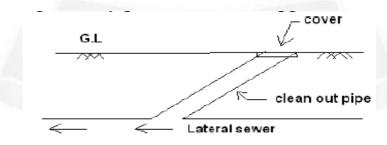
During blockage of pipe, the cover is taken out and water is forced through the cleanout pipe to lateral sewers to remove obstacles in the sewer line. For large obstacles, flexible rod may be inserted through the clean-out pipe and moved forward and backward to remove such obstacle.
