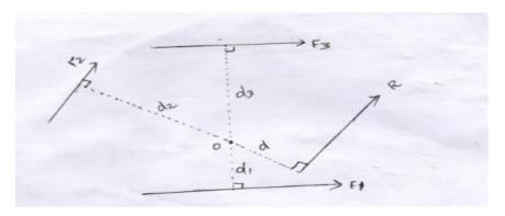
Find the resultant force for the parallel force System shown in fig.
