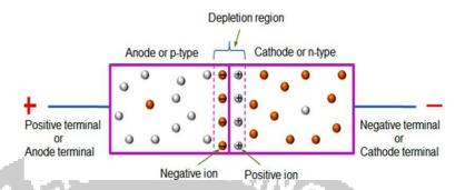
Cathode is the negatively charged electrode or conductor, which supplies free electrons to the p-n junction. In other words, cathode terminal or negative terminal is the source of free electrons, the negative charge carriers (free electrons) begins their journey at cathode terminal and travelthrough the diode and ends at anodeterminal.
