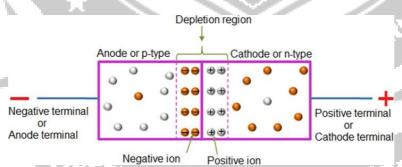
electrons from the negative terminal cannot move towards the positive terminal because the wide depletion region at the p-n junction resists or opposes the flow of freeelectrons.
