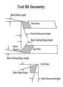
All the other angles are for clearance in order that no part of the tool besides the actual cutting edge can touch the work. The front clearance angle is usually 8 degrees while the side clearance angle is 10-15 degrees and partly depends on the rate of feed expected.
