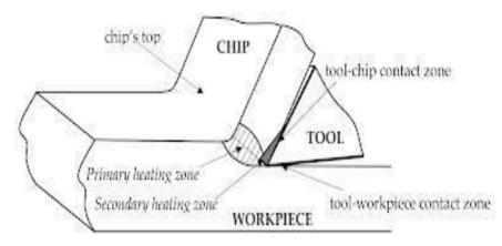
The cutting model shown above is oversimplified. In reality, chip formation occurs not in a plane but in so-called primary and secondary shear zones, the first one between the cut and chip, and the second one along the cutting tool face.
