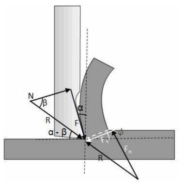
Forces acting on the chip on tool side and shear plane side
