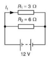
(a) The total circuit resistance R is given by 1/R = 1/R1 + 1/R2 = 1/3 + 1/6
