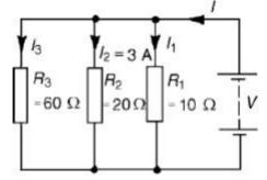
(a) P.d. across 20  $\Omega$ resistor = I2R2 = 3× 20 = 60V, hence supply voltage V =60V since the circuit is connected in parallel.
