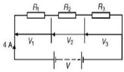
(a) Battery voltage V =V1 + V2 + V3 =5 + 2 + 6=13V (b)Total circuit resistance R= V/ I
