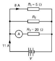
P.d. across R1 is the same as the supply voltage V. Hence supply voltage, V =8  $\times$  5=40V
