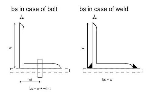
Lc - length of the end connection that is the distance between the outermost bolts in the end joint measured along the load direction or length of the weld along the load direction
