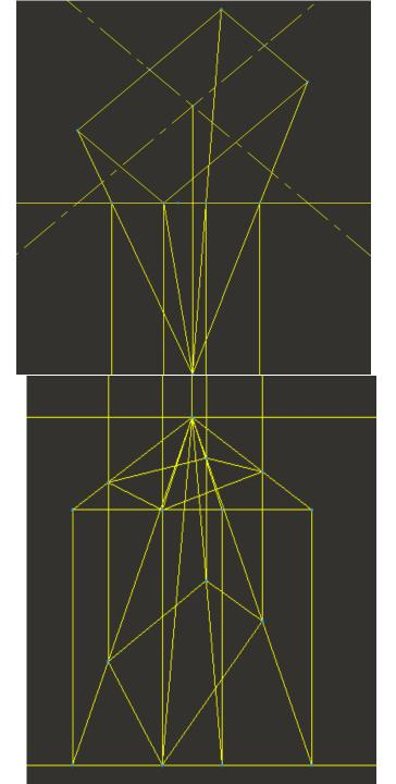
A rectangular lamina of size 30 mm x 50 mm rests on the ground with one edge on PP and the remaining portion behind PP. The station point is 60 mm above GP and 30 mm in front of PP and lies on a central plane 35 mm to the left of the nearest edge of the lamina. Draw the perspective view of the lamina. Univ qustn jan 13
