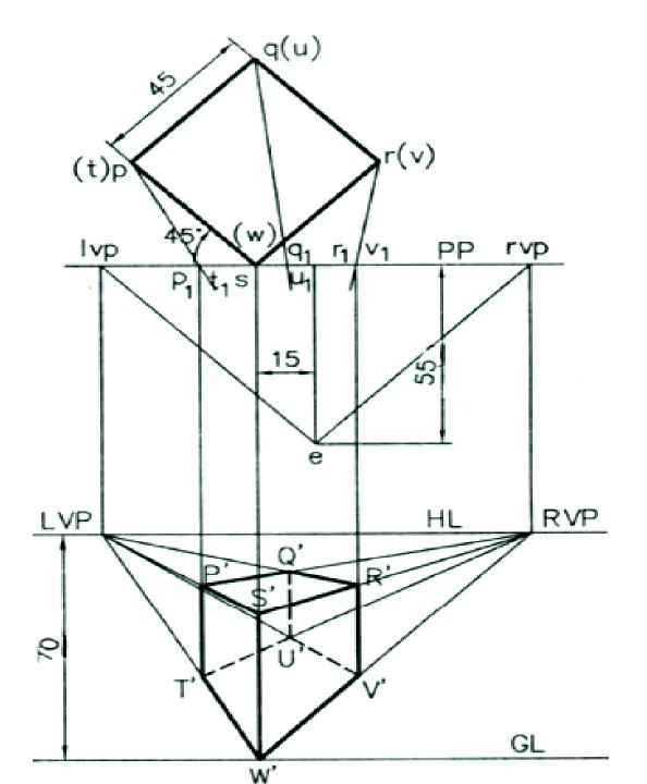
A triangular prism having an equilateral triangular base of sides 30 mm and height 40 mm rests on its base on the ground with one of its vertical edges 10 mm behind the PP. One of the rectangular faces containing that edge is inclined at 40° to the PP and is behind the PP. The station point is 50 mm in front of the PP and 50 mm above the ground. The station point is 15 mm to the right of the edge nearest to the PP. Draw the perspective projection of the prism. Page no 462
