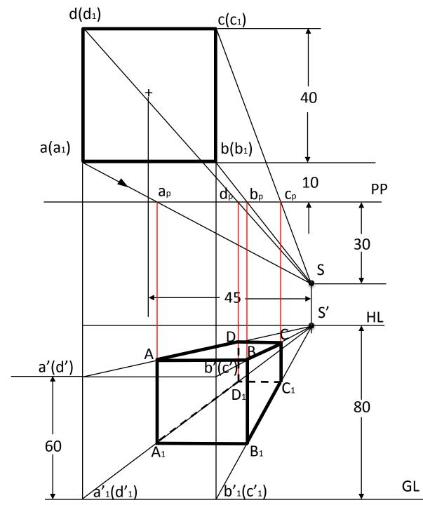
A square prism of base 25 X 25 mm and height 40 mm rests on the GP on one of its ends with a rectangular face receding away from the PP towards right making 60° with PP. The corner nearest to the PP is 40 mm to the left of the station point and 20 mm behind the PP. The station point is 60 mm above the GP and 50 mm in front of the PP. Draw the perspective view of the prism by visual ray method. Use the top view and the front view. Page no 432
