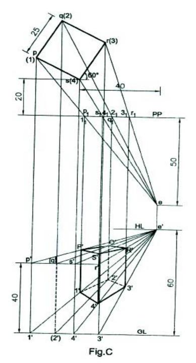
A rectangular prism sides of base 50 mm X 30 mm and height 55 mm rests with its base on the ground plane. A vertical edge is in the picture plane and one of the longer edges of its base is inclined at 45° to PP and behind it. The station point is 50 mm in front of PP, 75 mm above the ground plane and lies in a central plane which passes through the center of the prism. Draw the perspective projection of the solid. Page no 24.12
