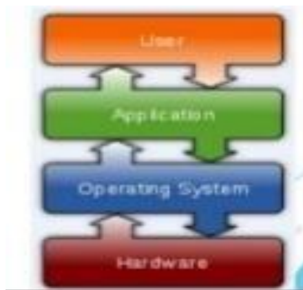
Layers of operating system
