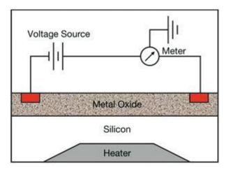
This image illustrates the working principle of a semiconductor gas sensor in a
