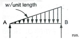
For numerical problem solving, the total UVL is converted into a point load as the area of the triangle and it acting at the C.G of the triangle. Take at a distance of 2/3 of total load acting from zero load.
