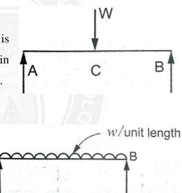
For numerical problem solving, the total UDL is converted into a point load acting at the centre of load.
