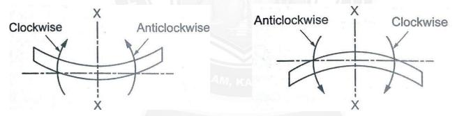
Similarly the bending moment at a section is considered negative if the bending moment at that section is such that it tends to bend the beam to a curvature haling convexity at the top. The negative B.M. as hogging Moment.
