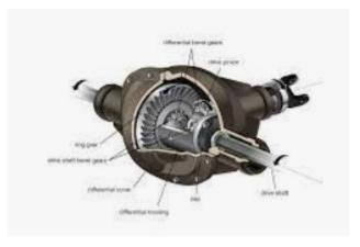
Each differential pinion can move in two planes simultaneously. When it is carried round by the casing, it drives the half shaft in the same direction but when it is rotated on its own shaft, it drives them in opposite direction i.e. rotation of differential pinion adds motion to one shaft and subtracts motion from the other shaft.
