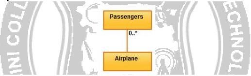
Multiplicity is the active logical association when the cardinality of a class in relation to another is being depicted. For example, one fleet may include multiple airplanes, while one commercial airplane may contain zero to many passengers. The notation 0..\* in the diagram means "zero to many".
