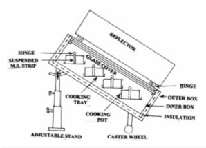
Fig-: Schematic Representation of Solar Cooker
