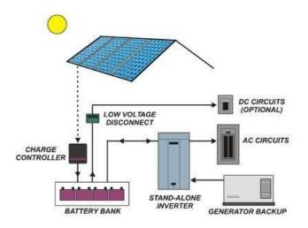
Fig-: Stand-alone roof top system with battery storage
