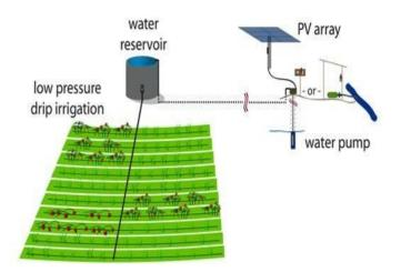
Fig-6: Solar water sprinkler- drip irrigation
