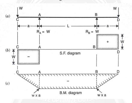
A beam simply supported at A and B and overhanging by same length at each support. A point load W is applied at each end of the overhanging portion. It is clear that there is no shear force between A and B but the B.M. between A and B is known as pure bending or simple bending.
