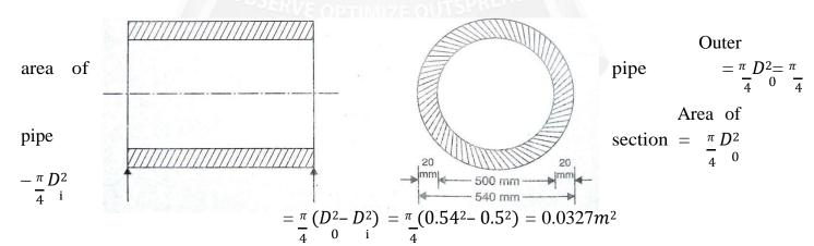
Moment of Inertia of pipe section about the neutral axis
