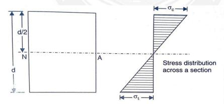
**Problem 3.1** A steel plate of width 120mm and of thickness 20mm is bent into a circular arc of radius 10m. Determine the maximum stress induced and the bending moment which will provide the maximum stress. Take  $E = 2 \times 10^5 N/mm^2$ .
