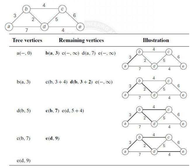
FIGURE 3.16 Application of Dijkstra's algorithm. The next closest vertex is shown in bold The shortest paths (identified by following nonnumeric labels backward from a destination vertex in the left column to the source) and their lengths (given by numeric labels of the tree vertices) are as follows:
