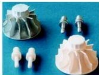
Investment casting of fan impeller from RP pattern
