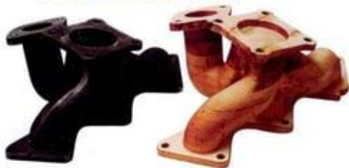
Cast metal (left) and RP pattern for sand casting (Courtesy of Helysis Inc.)
