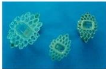
Investment casting of fan impeller from RP pattern
