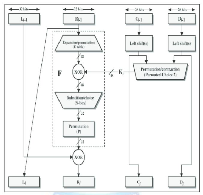
The round key Ki is 48 bits. The R input is 32 bits. This R input is first expanded to 48 bits by using a table that defines a permutation plus an expansion that involves duplication of 16 of the R bits. The resulting 48 bits are XORed with Ki. This 48-bit result passes through a substitution function that produces a 32-bit output, which is then permuted.
