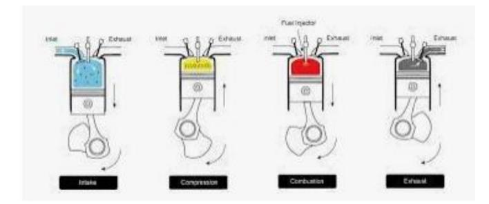
During the fuel injection period, the piston reaches the end of its compression stroke and commences to return on its third consecutive stroke, viz., power stroke. During this stroke the hot products of combustion consisting chiefly of carbon dioxide, together with the nitrogen left from the compressed air expand, thus forcing the piston downward. This is only the working stroke of the cylinder.
