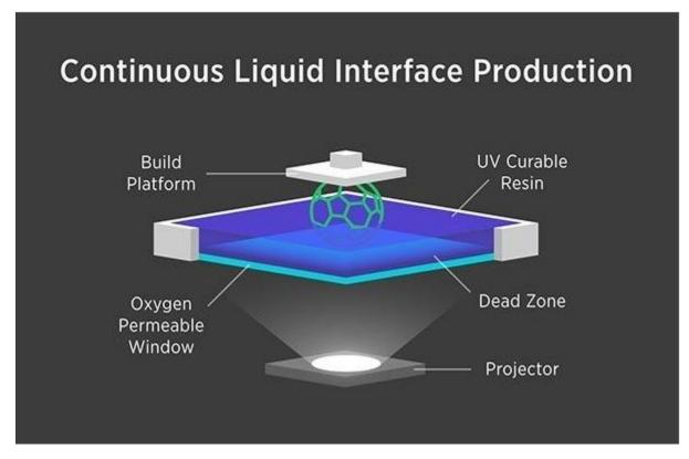
printers and their general arrangement, and we will use Figure to briefly explain the functionality of each part, starting from the bottom up.
