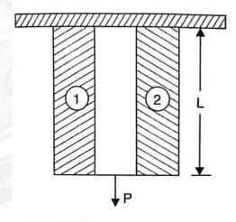
Now the total load on the composite bar is equal to the sum of the load carried by the two bars
