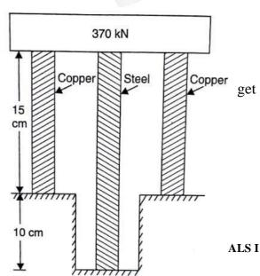
figure. The cross sectional area of steel rod is 2500 mm<sup>2</sup> and of each copper rod is 1600 mm<sup>2</sup>. Find the stresses in the rods. Take E for steel =  $2 \times 10^5$  N/mm<sup>2</sup> and for copper =  $1 \times 10^5$  N/mm<sup>2</sup>.
