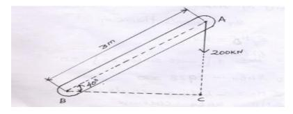
Vertical load at point A = 200KN
