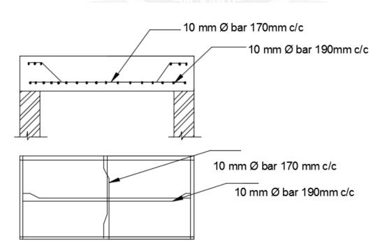
2.A slab has clear dimensions 3.5 m x 6 m with wall thickness 230 mm the live load on the slab is  $5 \text{ kN/m}^2$  and a finishing load of  $1 \text{kN/m}^2$  may be assumed. Using M20 concrete and Fe415 steel, design the slab
