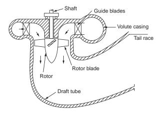
The number of blades depends on the head available and varies from 3 to 10 for heads from 5 to 70 m. As the peripheral speed varies along the radius (proportional to the radius) the blade inlet angle should also vary with the radius. Hence twisted type or Airfoil blade section has to be used. The speed ratio is calculated on the basis of the tip speed as  $\phi = u/\sqrt{2gH}$  and varies from 1.5 to 2.4. The flow ratio lies in the range 0.35 to 0.75.
