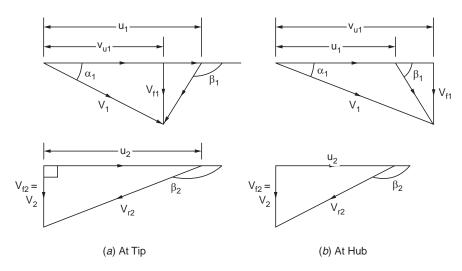
Figure 7.8.2 Typical velocity diagrams for Kaplan turbine
