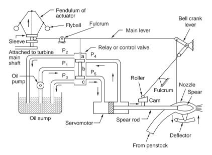
Figure 7.9.1 Governing system for Pelton turbine
