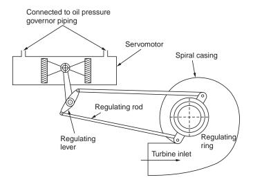
Figure 7.9.2 Reaction turbine governor linkage
