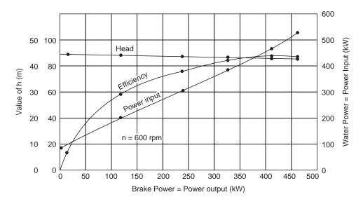
The efficiency curve is not as flat as that of impulse turbine. At part loads the efficiency is relatively low. There is a drop in efficiency after 100% load.
