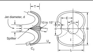
Figure 7.6.2 Pelton turbine bucket
