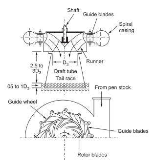
Figure 7.7.1 Typical sectional and front view of a modern Francis turbine.
