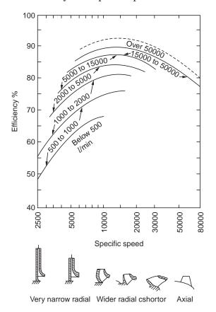
Figure 7.3.2 Variation of efficiency and flow passage with specific speed.
