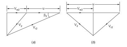
Figure 7.6.6 Exit velocity diagrams for pelton turbine
