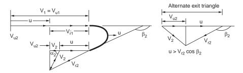
Figure 7.6.4 Velocity triangles Pelton turbine
