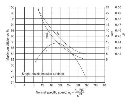
**Figure 7.6.10** Variation of efficiency at the  $\frac{D}{d}$  ratio for single jet inpulse turbine
