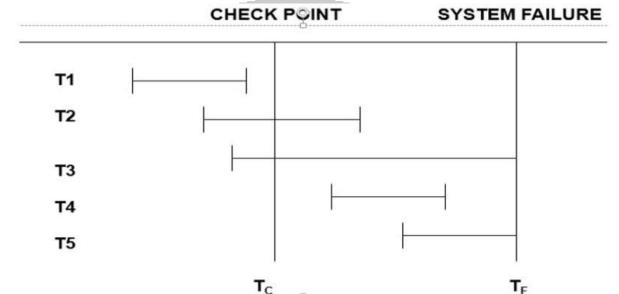
The system failure occurred at time Tf, the most recent check point prior to the time Tf was taken at a time Tc
