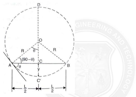
Let R = Radius of curvature of the deflected beam, y = Deflection of the beam at the centre (i.e., distance CC') I = Moment of inertia of the beam section,
