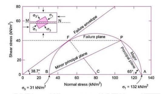
The Mohr's stress circle is so drawn that it is tangential to the envelope at point F.To do this, a line FC is drawn perpendicular to the envelope. With C as the centre and CF as the radius, a circle is drawn, which intersects the normal load axis at points A and B. Point A corresponds to the major principal stress  $\sigma$ 1 which comes out to be  $132 \text{kN/m}^2$  and point B corresponds to the minor principal stress  $\sigma$ 3 which Comes out to be  $31 \text{ kN/m}^2$  (31kPa).
