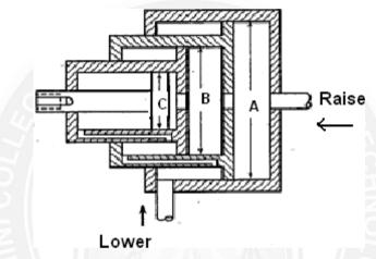
Since the diameter A of the ram is relatively large, this ram produces a large force for the beginning of the lift of the load. When ram A reaches the end of the stroke, ram B begins to move. Now ram B provides the required smaller force to continue raising the load. When ram B reaches the end of its stroke, then ram C moves outwards to complete the lifting operation. These three rams can be retracted by gravity acting on the load or by pressurized fluid acting on the lip of each ram.
