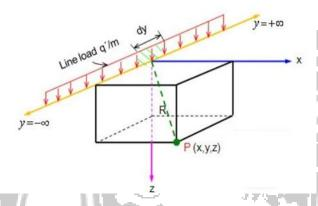
Let us consider the load acting on a small length dy. The load can be taken as a point load of q' dy using Boussinesq solution the vertical stress at P is given by
