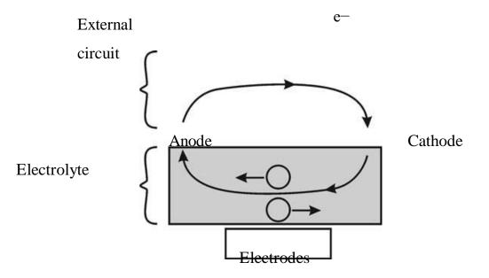
Figure: An electrode, a circuit for a cell which is converting chemical energy to electrical energy. The motion of negative charges is
