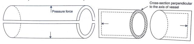
The forces, due to pressure of the fluid, acting at the thin cylinder, tend to burst the thin cylinder.
