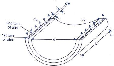
IF  $\sigma_w$  =Initial winding stress in wire
