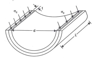
$\sigma_c$  = Compressive circumferential stress exerted by wire on cylinder =L $\times \frac{\pi}{2} \times d_w \times \sigma_w$
