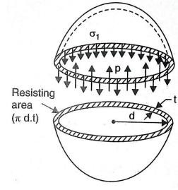
The stress  $\sigma_1$  is tensile in nature The fluid inside the shell is also having tendency to split the shell into two hemispheres along y-y axis. Then it can be shown that the tensile hoop stress will also be equal to  $\frac{pd}{4t}$ . Let the stress is  $\sigma_2$
