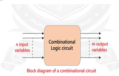
The 'n' input variable comes from the external source while the 'm' output variable goes to the external destination. In many applications, the source or destinations are storage registers.
