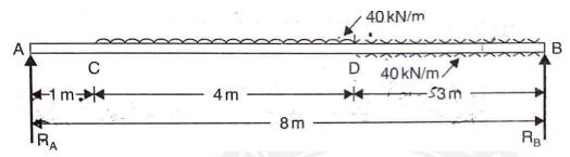
BM for the section X-X is given by,
