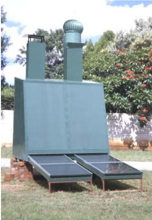
Passive cabinet solar dryers
