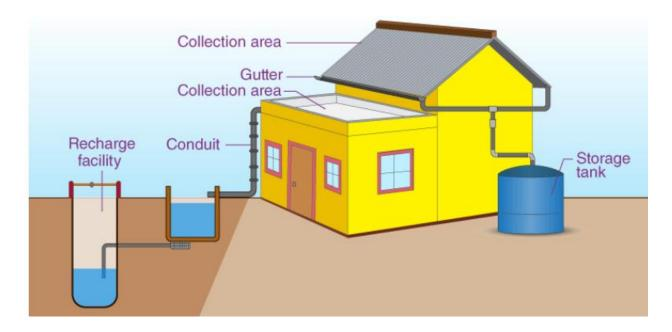
Rainwater harvesting systems consists of the following components:
