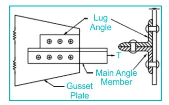
The lug angle serves as a compact angle piece strategically employed to link the outstand legs of members to the gusset plate in steel structures. Its primary objectives are to minimize the overall length of the connection to the gusset plate and mitigate the shear lag effect. This essential structural element contributes to the efficiency of connections by streamlining design and optimizing load-bearing capabilities.
