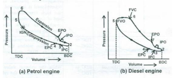
Figure P-V diagram of two stroke cycle engine
