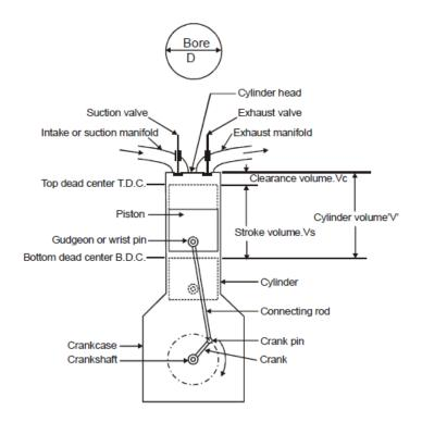
Figure 3.1 Cross section of an Internal Combustion Engine
