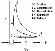
Figure Actual P-V diagram of four stroke Otto cycle engine
