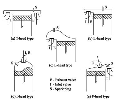
The different types of combustion chamber used in SI engine are
