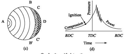
Combustion with detonation
