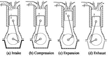
**Figure Four Stroke Cycle SI Engine**
