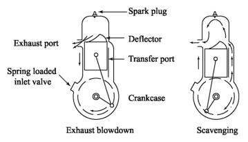
Figure Two stroke cycle engine
