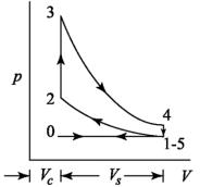
Figure Theoretical P-V diagram of four stroke Otto cycle engine
