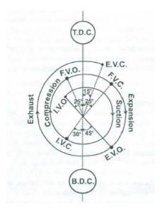
Actual valve timing diagram of CI engine
