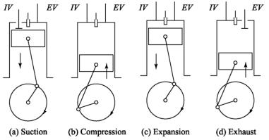
**Figure Four Stroke Cycle CI Engine**
