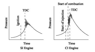
The phenomenon is similar to that in the SI engine. However, in the SI engine knocking occurs near the end of combustion whereas in the CI engine knocking occurs near the beginning of combustion. In order to decrease the tendency of knock it is necessary to start the actual burning as early as possible after the injection begins. In other words it is necessary to decrease the ignition delay and thus decrease the amount of fuel present when the actual burning of the first few droplets starts.
