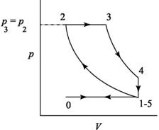
Figure Theoretical P-V diagram of four stroke Diesel cycle engine
