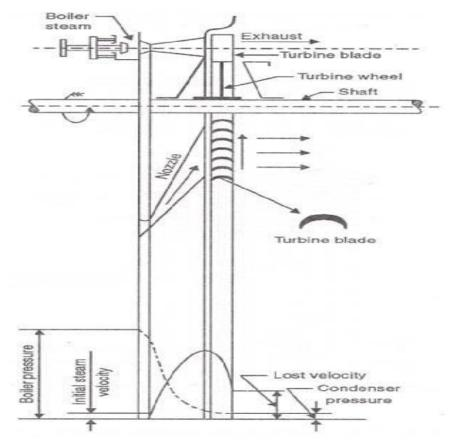
An impulse turbine runs by the impulse of steam jet. In this turbine the steam isfirst made to flow through a nozzle. Then the steam jet impinges on the turbine blades. The steam jet after Impinging on the rotor blades glides over the concave surface of the blades and finally Leaves the turbine.
