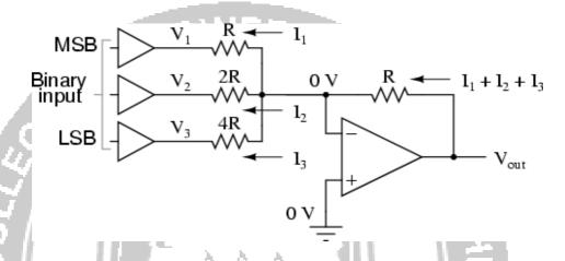
If we chart the output voltages for all eight combinations of binary bits (000 through 111) input to this circuit, we will get the following progression of voltages:
